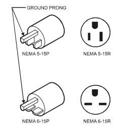
Fig. 3 Electrical Plug and Receptacle Configuration
